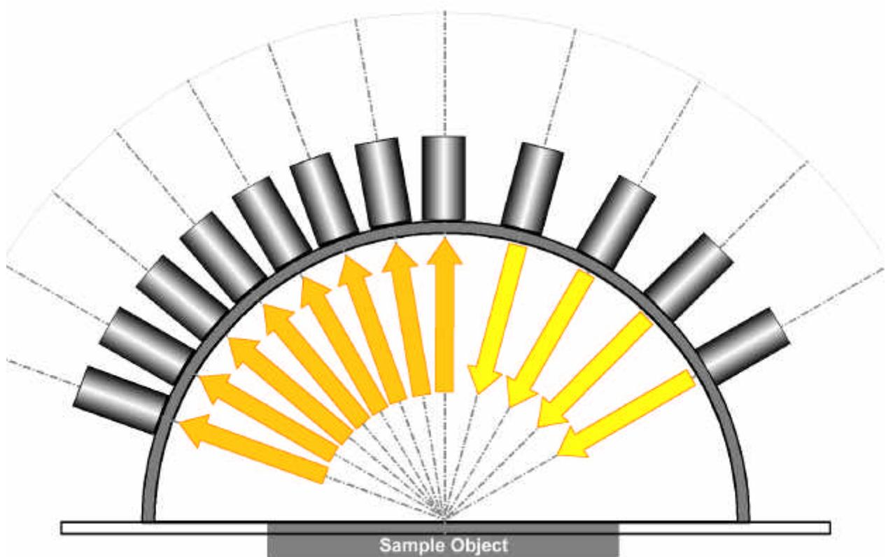
**Figure 1:** Typical example for a measurement head with 4 illuminating and 8 reflected beams at various inclinations, in-plane configuration, light-guiding fibers not shown (see Fig. 2).
